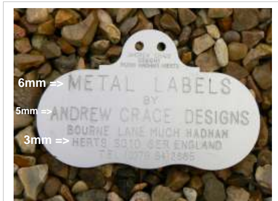
Sample of label punched with 3 different sizes of Alitags character punches, i.e. 6mm, 5mm and 3mm
